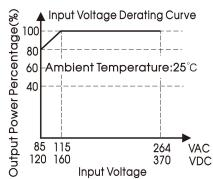
Note: ① With an AC input between 85-115VAC and a DC input between 120-160VDC, the output power must be derated as per temperature derating curves; ② This product is suitable for applications using natural air cooling; for applications in closed environment please consult factory or one of our FAE.
